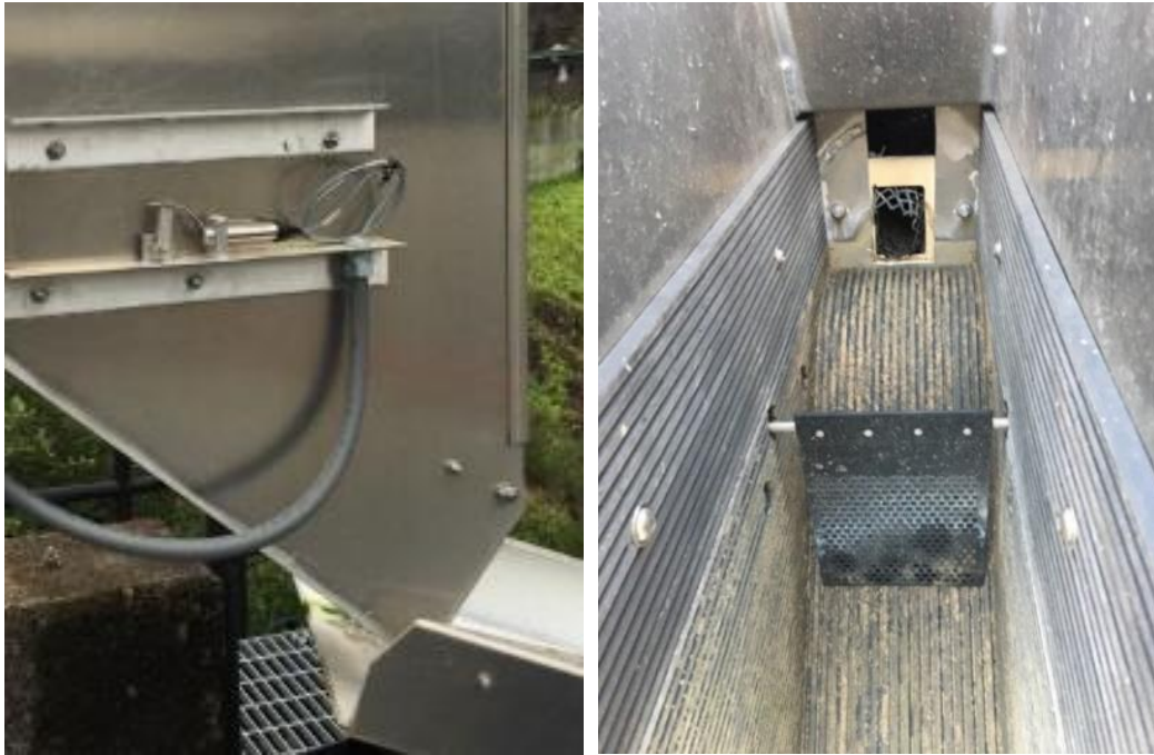
Figure 3. Bradford Island LPS mechanical counter components new for 2018. Left, proximity detector and ferrous tab (cover removed). Middle, inside of camera box showing black paddle, 1/8" grooved PVC, upwelling box fyking, and smooth face near the fyking where some lamprey attached. Not shown Dwyer counter display and DATAQ DI-161 data logger installed in the count station.
